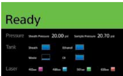
The LCD monitor on the front of the SH800 displays status information during operation.
